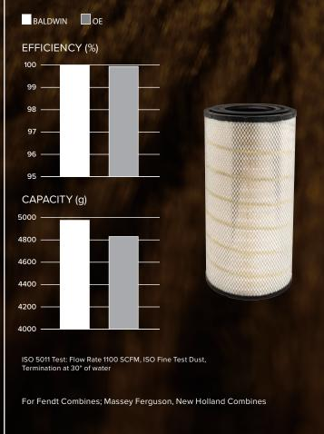
Baldwin filters are vigorously tested above and beyond industry standards, ensuring reliable performance under the toughest conditions.
