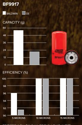
ISO 19438 Test: Flow Rate 3 gpm, ISO Medium Test Dust,  $104^\circ\text{F},$  Termination at 5 psid
